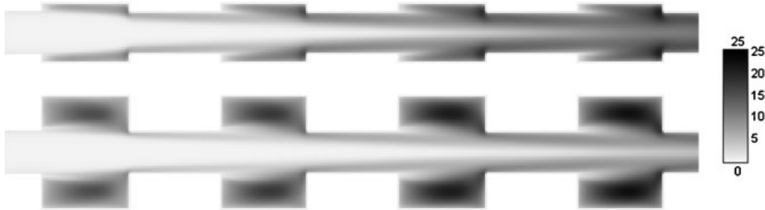
Figure 10. 2D turbulent viscosity components ( 10 \times 4 \text{ m}^2/\text{s} ) in the upstream part of the macro-rough channel reach ( 7.50 \text{ m} < x < 14.9 \text{ m} ). Configuration 221 (up) and 224 (down) with specific discharge q_4 .
